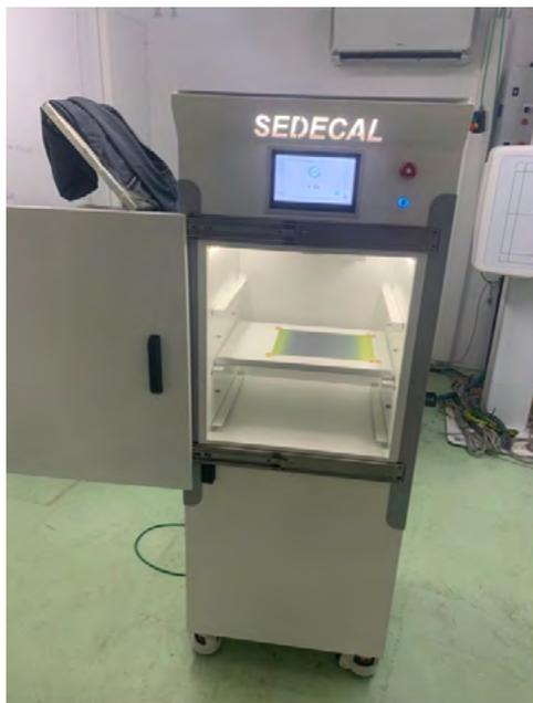
Figure 1. Prototype of the X-ray irradiator
